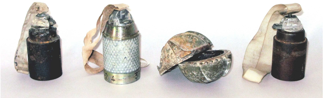
Cluster bomb submunitions. From left to right: M42/M46, MZD2, BLU-63 and M77 (Photo © DanChurchAid/Jawad)
