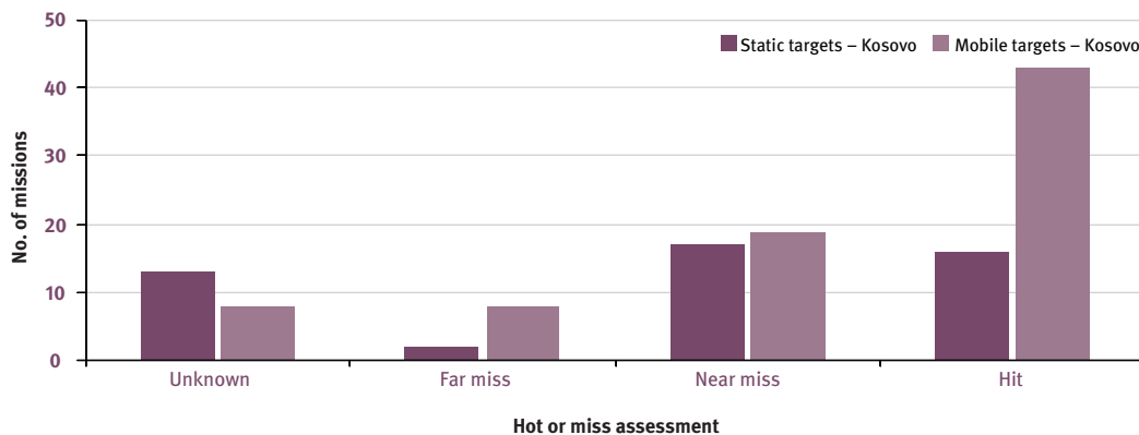
Hit or miss assessment of RBL755 missions against static targets in Kosovo with strikes on mobile targets for comparison
